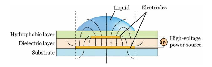
Principle of PLEEC. An asymmetric capacitor is separated by a dielectric layer. Credit: Science Advances, doi: 10.1126/sciadv.aau8769
