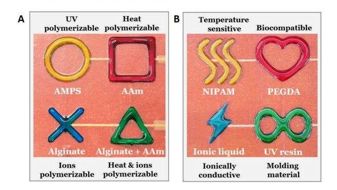
(A) Liquid patterns of four representative hydrogel precursors with different chemical and physical properties and polymerization into hydrogel via different polymerization methods. (B) Liquid patterns of four functional materials: temperature sensitive, biocompatible, ionically conductive, and molding materials. Photo credit: Jikun Wang, Xi'an Jiaotong University. Credit: Science Advances, doi: 10.1126/sciadv.aau8769
