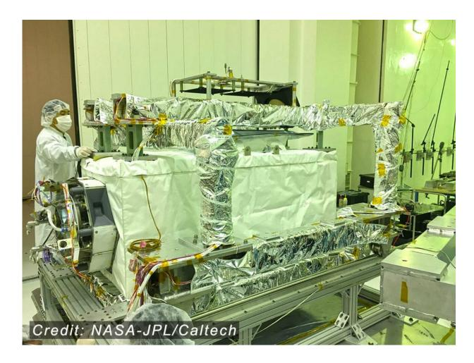
The ECOSTRESS instrument is housed in a large box that plugs into the outside of the International Space Station. Here, the instrument is seen in development at NASA's Jet Propulsion Laboratory prior to launch. Credit: NASA-JPL/Caltech
