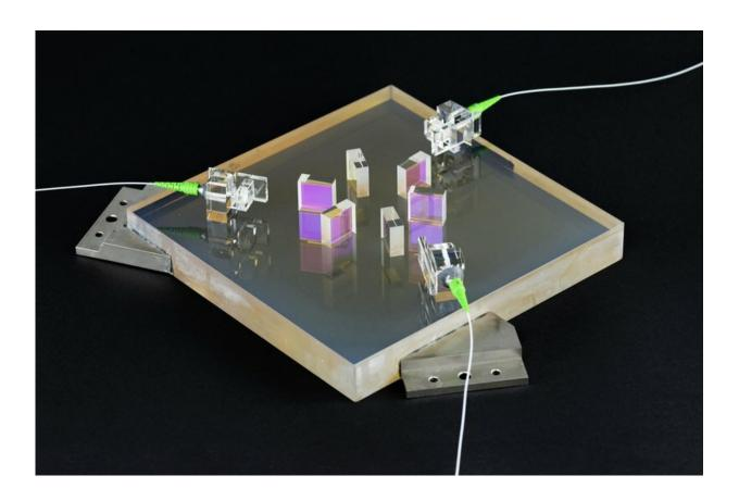
The AEI Hannover optical bench for test of LISA technology before it was integrated in the vacuum chamber. The three lasers are transmitted via optical fibres. Credit: D. Penkert/Max Planck Institute for Gravitational Physics
