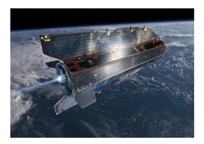
In orbit, the same side of the GOCE satellite remains facing the Sun. The spacecraft is equipped with four body-mounted and two wing-mounted solar panels. Due to the configuration in orbit, the solar panels will experience extreme temperature variations so it was necessary to use materials that will tolerate temperatures as high as 160°C and as low as -170°C. Credit: ESA–AOES-Medialab
