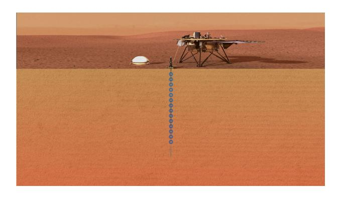
GB: RAD radiometer of HP3 for measurements of surface temperature. Supplements temperature data at depth for a long-term measurement of the temperature over a period of up to two years. 14 sensors are soldered at approximately 35-centimetre intervals onto the science tether. Credit: DLR German Aerospace Center
