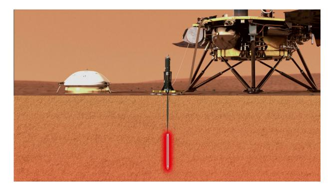
GB: The "Mole" measures the thermal conductivity of teh soil approximately every 50 centimetres up to a depth of 5 meters. Credit: DLR German Aerospace Center
