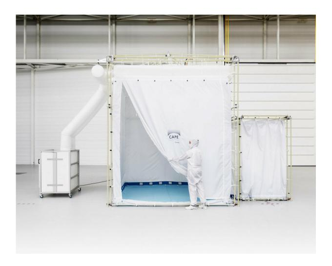
CAPE is as flexible as a tent, providing an ultra-clean manufacturing environment that complies with air cleanliness standards all the way up to ISO class 1. Credit: Fraunhofer IPA/Rainer Bez
