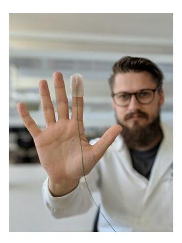
A new wearable probe enhances the sense of touch by imaging and quantifying the stiffness and elasticity of biological tissue. The device could help improve the surgical removal of breast cancer and other types of cancer. Credit: Rowan W. Sanderson, University of Western Australia
