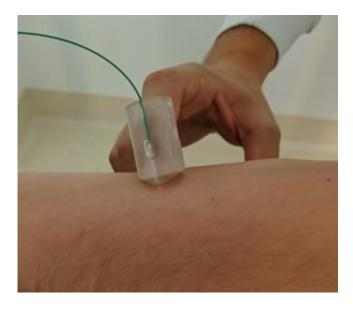
To use the device, the finger-mounted probe is placed perpendicular to the body and pressed on the tissue while OCT images are recorded. The researchers want to incorporate the sensor into a surgical glove that would preserve touch sensitivity. Credit: Rowan W. Sanderson, University of Western Australia
