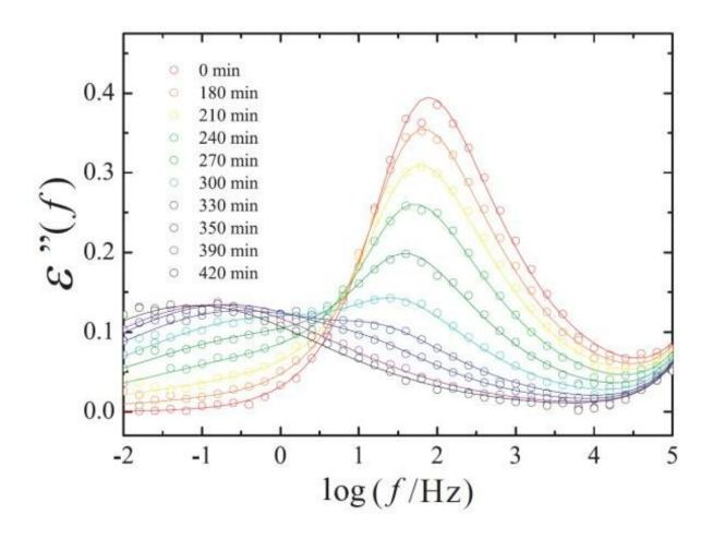
Time evolution of dielectric loss spectra during liquid-liquid transition of triphenyl phosphite at 214 K. The horizontal axis is the measurement frequency. The frequency of the peak shifts to lower frequencies with time, the dynamics of liquid is drastic slowing down of with liquid-liquid transition. Credit: 2019 Hajime Tanaka, Institute of Industrial Science, The University of Tokyo
