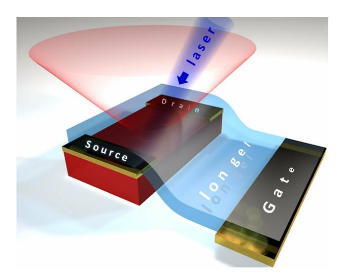
Conceptual view of a transistor device that controls photoluminescence (the light red cone) emitted by a hybrid perovskite crystal (the red box) that is excited by a blue laser beam after voltage is applied to an electrode (the gate). Credit: Vitaly Podzorov and Yaroslav Rodionov
