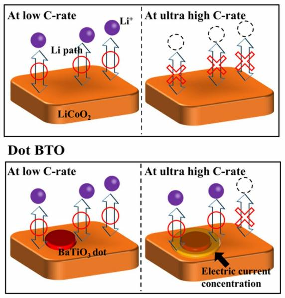
The  $BaTiO_3$  nanodots concentrate electric current in a ring around them and create paths through which Li ions can pass, even at really high charge/discharge rates. Credit: Nano Letters
