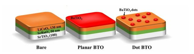
Three cathodes were fabricated: a standard bare one (left), one coated with a layer of  $BaTiO_3$  (middle), and one coated with several  $BaTiO_3$  nanodots (right). The one with the nanodots exhibited greatly enhanced performance. Credit: Nano Letters
