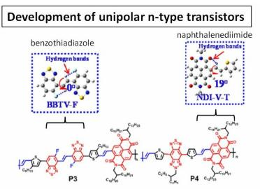
1. Improved coplanarity of polymer backbones via intramolecular hydrogen bonds
