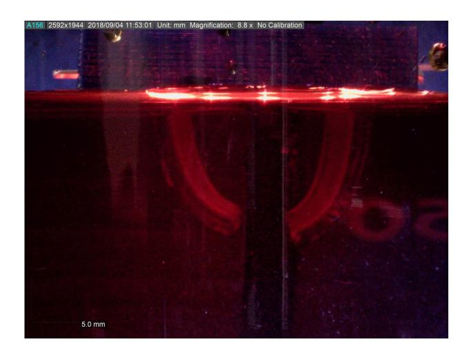
A new hydrogel material is able to respond dynamically to its environment. In the presence of iron ions, the material bends on its own, in this case to close a gripper that can pick up small objects Credit: Wong Lab / Brown University
