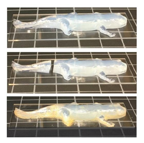
A new kind of hydrogel material developed at Brown has the ability to react dynamically to its environment--bending, twisting and self-adhering on demand. Above, the researchers demonstrated self-adhering behavior on the tail of a 3-D printed hydrogel salamander. The self-adhering behavior was also used to make hydrogel building blocks that fit together like LEGO blocks. Credit: Wong Lab / Brown University
