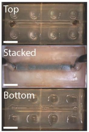
LEGO-like hydrogel building blocks patterned with tiny fluid channels can be assembled into complex microfluidic devices and then sealed tightly together. Credit: Wong Lab / Brown University
