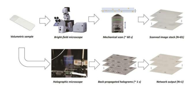
Bright-field Holography (BH): a novel technique for high contrast microscopic object imaging in sample volumes. Credit: UCLA Engineering Institute for Technology Advancement
