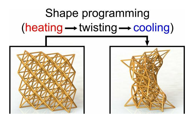
4D-printed metamaterials can be temporarily transformed into any deformed shape and then returned to their original shape on demand when heated. The scale bar is 2 millimeters. Credit: Chen Yang/Rutgers University-New Brunswick
