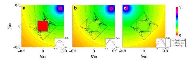
Simulated equipotential line patterns under different hidden objects or positions. The center object with a square insulator, b circular conductor, and c when the source is placed at a different location. Credit: Light: Science & Applications, doi: 10.1038/s41377-019-0141-2
