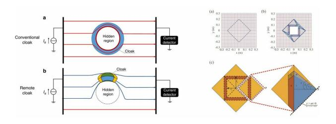
Left: Schematics of two kinds of DC cloaking. a) Conventional cloaking and b) remote cloaking. Right: The schematic of the transformation applied. (a) Meshes for the virtual space with background media. (b) Meshes for the physical space after defined multi-folded transformation. (c) The schematic of the transformation from the conventional square cloak to the remote cloak. Credit: Light: Science & Applications, doi: 10.1038/s41377-019-0141-2
