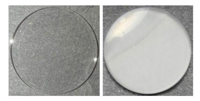
The small sapphire disk on the right shows organic aerosols formed inside a high-temperature oven. The disk to the left has not been used. Credit: NASA/JPL-Caltech
