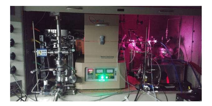
JPL scientists used the "oven" (center) to heat a mixture of hydrogen and carbon monoxide and subject it to UV radiation, generated by a hydrogen gas discharge lamp. The lamp radiates both visible light (the pink glow) and UV light, which enters the gas container inside the oven via a window on the right side. Credit: NASA/JPL-Caltech
