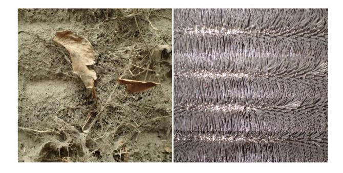
Close-up of 17 grams of dirt per square foot on an air conditioner condenser and that same condenser after it's cleaned. Credit: Mehdi Mehrabi, <u>CC BY-SA</u>
