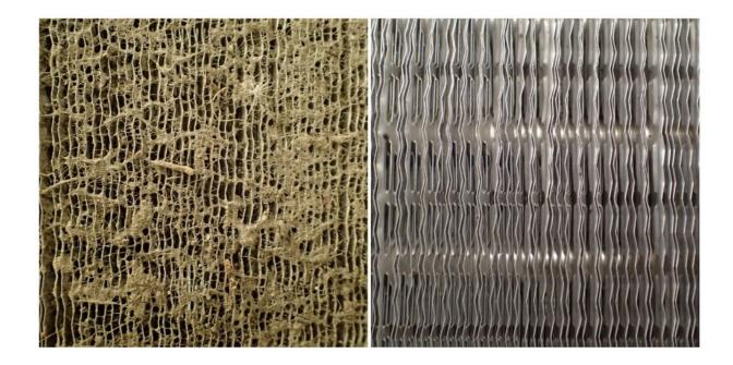
Close-up of 7 grams of dirt per square foot on an air conditioner condenser and that same condenser after it's cleaned. Credit: Mehdi Mehrabi, <u>CC BY-SA</u>
