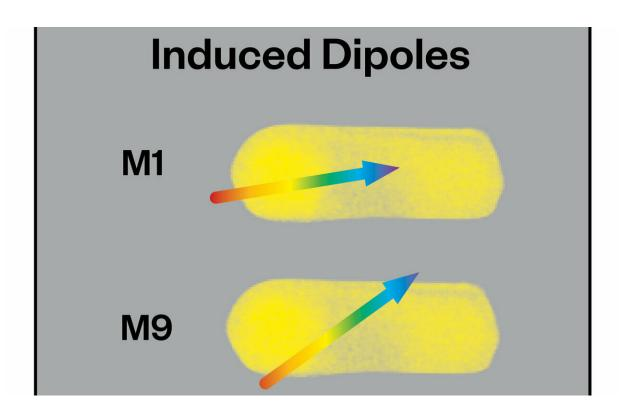
Illustration shows the process of using dipoles induced by specific molecules to measure their damping effect on gold nanoparticle plasmons. Credit: Alese Pickering/Rice University
