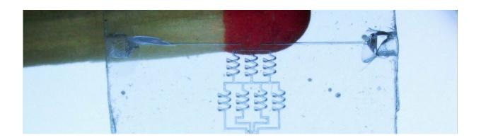
Three-dimensional hollow structures in quartz glass. Credit: AG Rapp
