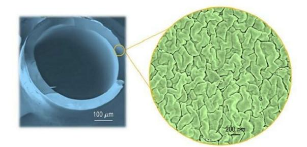
The team created well-formed cellulose hollow-fiber membranes for separating oil-in-water mixtures. Credit: KAUST
