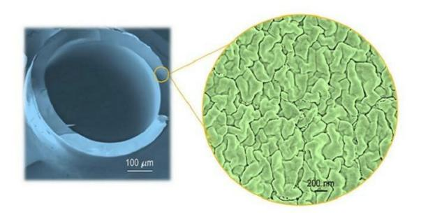
The team created well-formed cellulose hollow-fiber membranes for separating oil-in-water mixtures. Credit: KAUST
