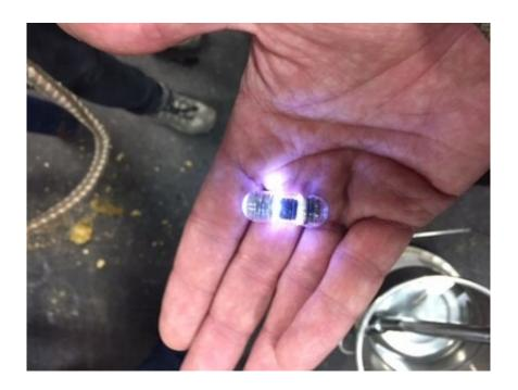
The capsule has four cameras, a LED light source, and an on-board video recording system with a motion detection system. Credit: Renaud Léguillette
