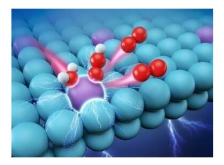
Ru was atomically dispersed in metal support. In acidic electrolyte environment, water molecules was adsorbed on the active site Ru atom under the applied potential, and then single atom Ru catalyst boosts acidic water electrolysis producing oxygen via OOH mechanism. (Purple, blue, red and white balls represents Ru, Pt, O and H atoms, respectively.) Credit: WU Yuen
