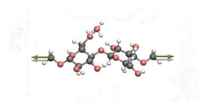
The molecular structure of cellulose, to which nanoscientists applied mechanical force (green arrows). The hydrolysis reaction changed dramatically as a result. Credit: Saeed Amirjalayer et al./Angew Chem
