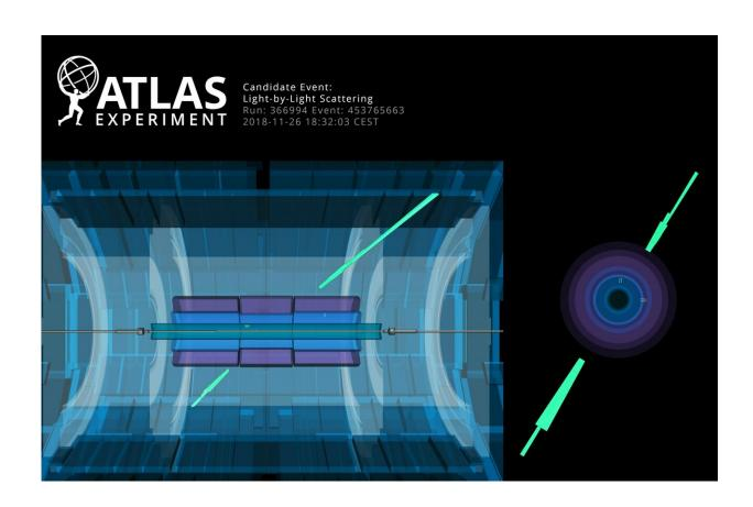
ATLAS event display showing the energy deposits of two photons in the electromagnetic calorimeter (green) on opposite sides and no other activity in the detector, which is the clean signature of light-by-light scattering. Credit: ATLAS Collaboration/CERN
