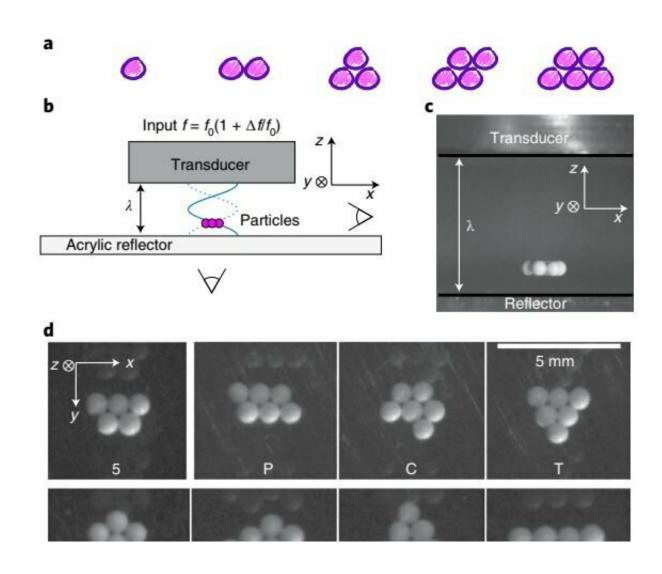
Assembling and manipulating clusters composed of macroscopic particles using acoustic levitation. a, Sketches of compact cluster configurations (isostatic ground states) for one to five particles. b, Schematic of the experimental set-up. An ultrasound transducer generates sound waves in air, with speed of sound cs=
