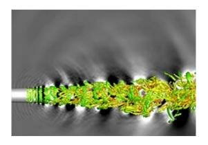
Turbulent flow structures with noise shown at the background. Credit: Zhi Wang.
