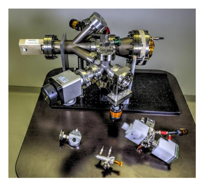
This image shows the Modulated X-ray Source, a key component in NASA's first-ever demonstration of X-ray communication in space. Credits: NASA/W. Hrybyk
