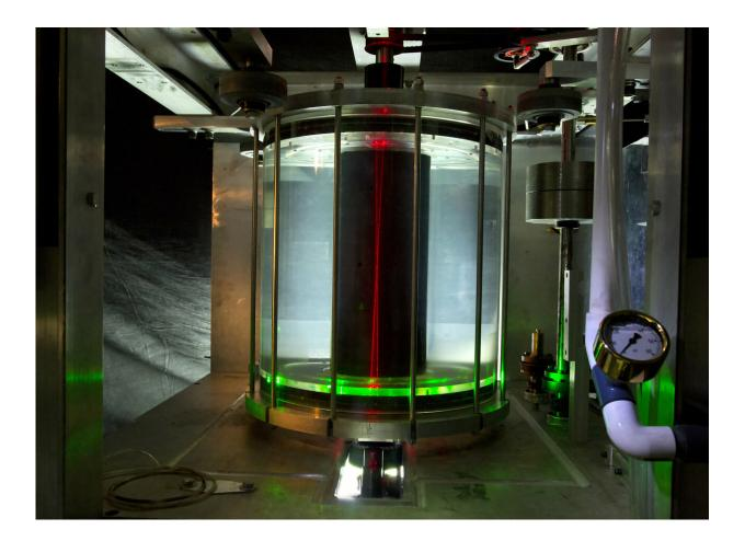
Water-filled version of MRI experiment showing transparent outer cylinder and blackened inner cylinder. Red lasers enter at bottom to measure the local speed of the water. Credit: Eric Edlund and Elle Starkman
