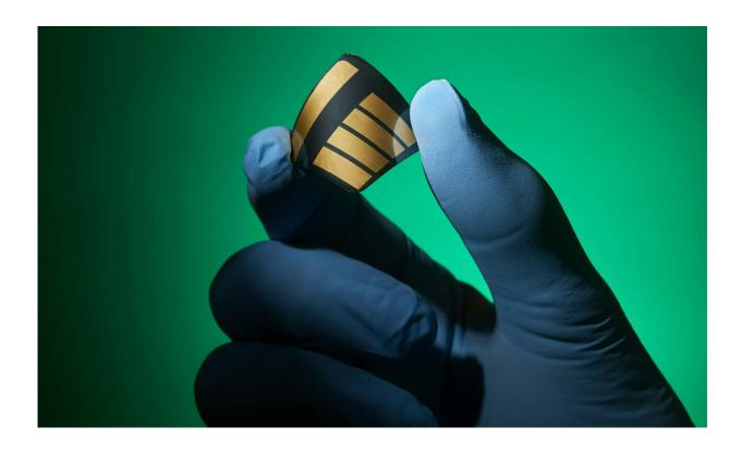
Solar cells made of perovskite have great promise, in part because they can easily be made on flexible substrates, like this experimental cell. Credit: Ken Richardson
