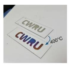
A thermally painted subwavelength metasurface produces a dazzling array of colors that do not change with viewing angle. Am oxide layer that is a few nanometers thick was grown at the edge of the metal at high temperatures. This created the optical metasurface that perfectly absorbs certain wavelengths of light. Credit: Giuseppe Strangi, Case Western Reserve University
