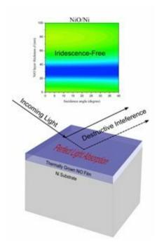
Perfect light absorption occurs in the nickel oxide (NiO) metasurface because light rays emerging from the oxide layer and the metal substrate come together in such a way that they cancel each other out – a phenomenon known as total destructive interference. Credit: Giuseppe Strangi, Case Western Reserve University
