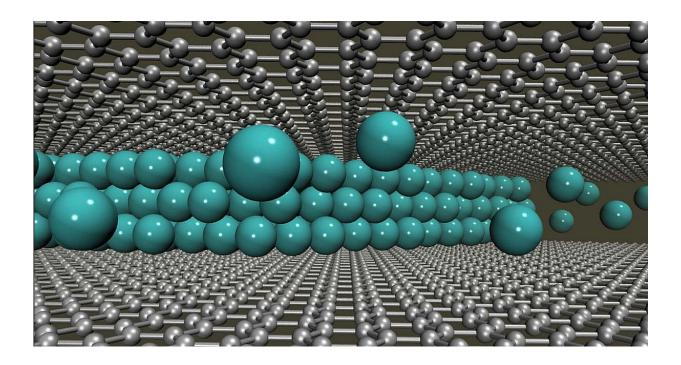
Atomistic model illustrating a multilayer of lithium atoms between two graphene sheets. Credit: Dr. Mahdi Ghorbani-Asl, HZDR. See M. Kühne, et al., *Nature* 564 (2018).
