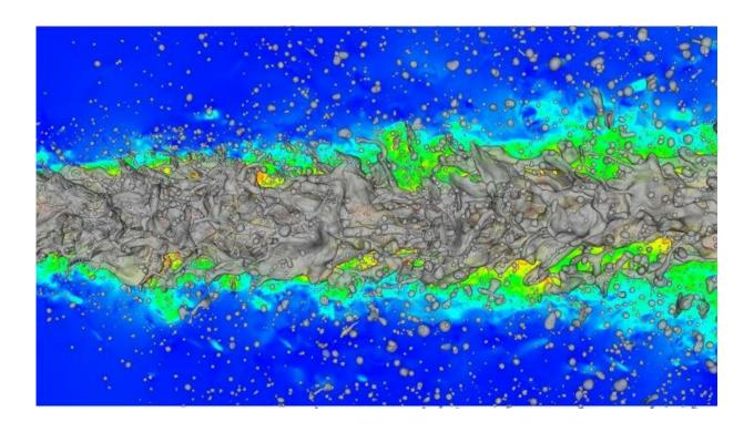
Visualization of the liquid surface and velocity magnitude of a round jet spray. Credit: Bundeswehr University Munich
