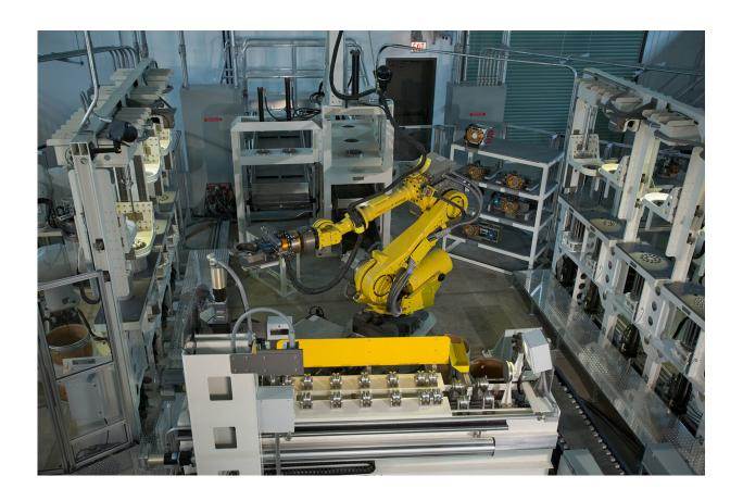
This automated system demilitarizes warheads by cutting them into separate sections, removing foam packs filled with grenades and detaching grenade fuses. Credit: Regina Valenzuela
