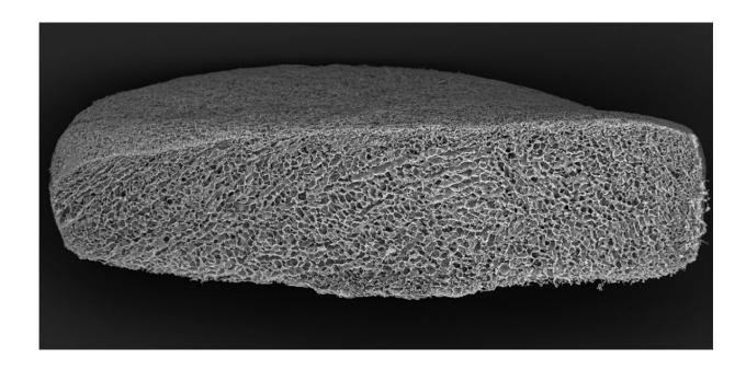
An SEM cross-section of the injectable sponge, showing pore shape and structure. Scale bar, 200 nanometers. Credit: Harvard University
