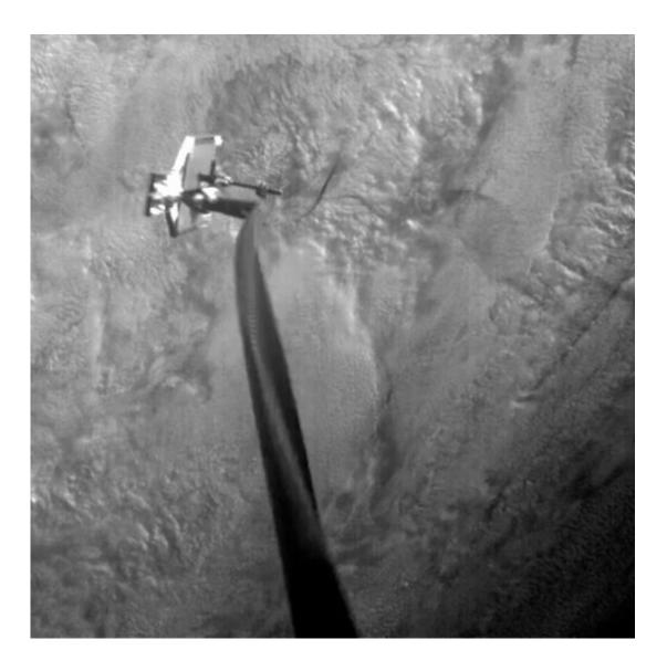
This Feb. 8, 2019 image from video made available by the RemoveDEBRIS Consortium shows a harpoon striking a square target mounted 1.5 meters (5 feet) from the RemoveDEBRIS spacecraft. The same team used a net to capture a
