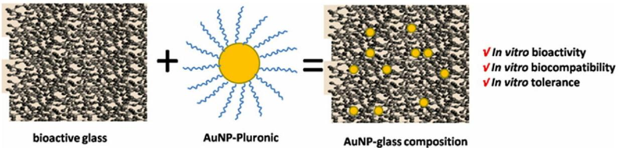
The gold nanoparticles embedded in silicate bioactive glasses prepared by the sol-gel method. Image credit: Materials Science and Engineering: C, Credit: Biomedical Materials, doi: <https://doi.org/10.1088/1748-605X/aafd7d>
