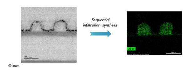
TEM image of the photoresist pattern after lithography exposure (left) and TEM EDX signal from Aluminum for the photoresist pattern after the SIS step (right). Credit: IMEC
