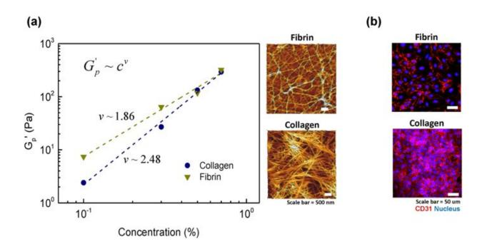
Analysis of chain flexibility of hydrogel: (a) power-law scaling of plateau modulus with a concentration of hydrogel for collagen and fibrin. Dash lines are the results of fits to power law equation G'p=cv and microstructure of two representative samples of 0.5% concentration each in collagen and fibrin. (b) cell
