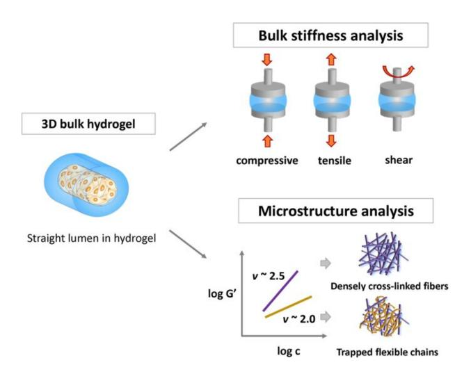
Schematic representation of methods for characterizing the physical properties of hydrogel: the bulk stiffness of hydrogel and chain flexibility in viscoelastic networks through the semi-flexible model. Credit: *Scientific Reports*, doi: https://doi.org/10.1038/s41598-019-38951-7
