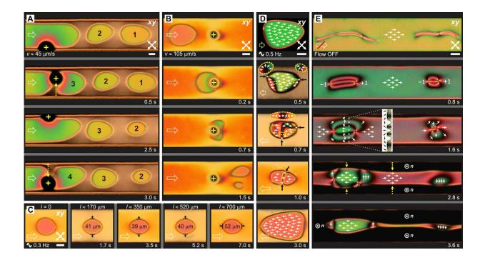
Systematic reshaping of dowser domains under laser action and oscillatory flows. (A) Moving the laser beam transversely across the bulk dowser pinches off a uniform "train" of the domains. (B) A static beam at a low power of 80 mW generates a small isotropic region that cuts a large dowser domain longitudinally in half. (C) The shape and size of the domain can be maintained over long time and length scales by periodically modulating the driving pressure around the
