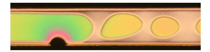
Producing a steady stream of dowser domains by chopping the bulk dowser state with a moving laser spot. By moving an isotropic island of laser-heated nematic phase transversely across the phase boundary between the dowser and bowser state (black) one can produce a uniform train of dowser domains. Recorded under crossed polarizers at 30 fps, the view field size is 480  $\mu$ m × 120  $\mu$ m. Credit: Science Advances, doi: 10.1126/sciadv.aav4283
