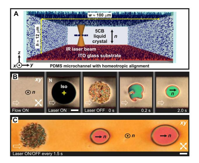
Nucleation of orientation phase domains in pressure-driven nematic microflows. (A) Schematic illustration of a channel with homeotropic anchoring on the top and bottom surfaces used in the experiment; IR, infrared; ITO, indium tin oxide. (B) The nematic in a channel looks black between crossed polarizers in the absence of flow and gains visible birefringence due to flow-driven director distortion that traps a domain of the flow-aligned state (also called the dowser
