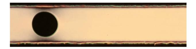
Expansion and contraction of laser-nucleated dowser domains in a moderate nematic microflow. The lifetime of the domain is proportional to the critical velocity and the initial size. Recorded under crossed polarizers at 30 fps, the view field size is 480  $\mu$ m × 120  $\mu$ m. Credit: Science Advances, doi: 10.1126/sciadv.aav4283
