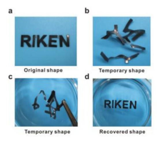
a. A film was cut into a RIKEN logo and painted, (permanent shape at 20 °C). b. The RIKEN-shaped sample was deformed at 50 °C and the deformed temporary shape was fixed by cooling to 20 °C. c. The deformed temporary shape was
