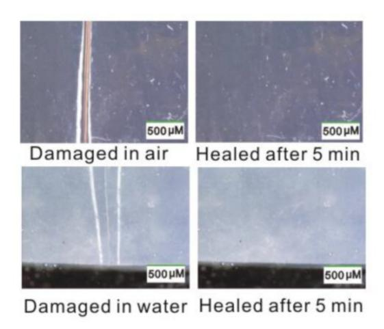
Top panel: Optical microscope images of damaged (left) and repaired (right) samples of one of the materials in air at 25 °C. A film was cracked by razor blade and then left in air for 5 minutes for healing. Bottom panel: Optical microscope images of damaged (left) and repaired (right) samples of one of the films in water at 25 °C. The film was cracked by a razor blade and then left in water for 5 minutes for healing. Credit: RIKEN
