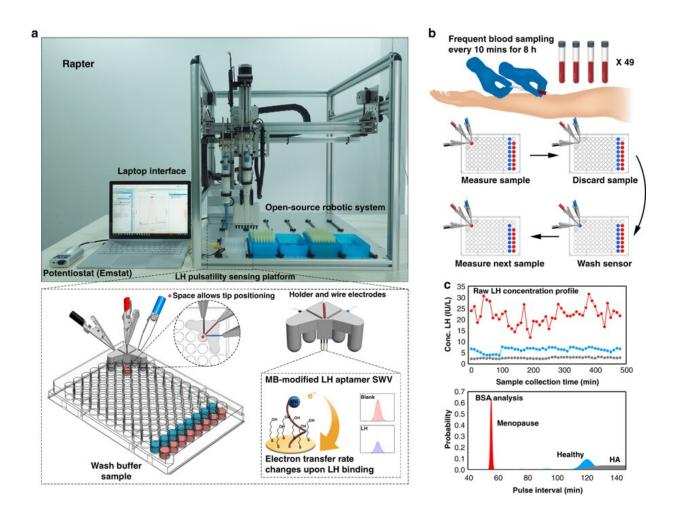
Overview of the Robotic APTamer-enabled electrochemical reader (RAPTER). a RAPTER design. RAPTER consists of a potentiostat, laptop interface, opensource liquid-handling robot and the 96-well-plate sensing platform. The quantification of the LH level is achieved by analysing the electron transfer kinetic changes (interrogated via square-wave voltammetry (SWV)) upon binding of LH under a three microwire electrode system held within a 3D-
