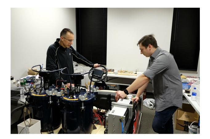
Eric Nauman, professor in mechanical engineering and in basic medical sciences and co-founder of IFBattery, and Michael Dziekan, senior engineer for IFBattery, run tests on a membrane-free, flow battery being used to power a golf cart. The battery has the potential to generate enough energy to drive an electric car up to 3,000 miles. Credit: Lyna Landis, Purdue Research Foundation
