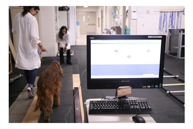
The author walks a dog across the pressure-sensitive walkway with Dr. Romany Pinto at the end of the walkway to keep the dog focused ahead. To obtain optimal gait data, the animal must walk in as straight a line as possible on the walkway, without turning its head or pulling on the lead. The computer screen shows the animal's footsteps as they occur on the walkway. Credit: Emma Thomson
