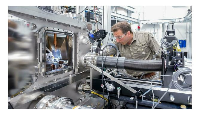
Argonne nanoscientist Martin Holt took X-ray images of the acoustic waves with the Hard X-ray Nanoprobe at the Center for Nanoscale Materials and Advanced Photon Source, both at Argonne. Credit: Argonne National Laboratory
