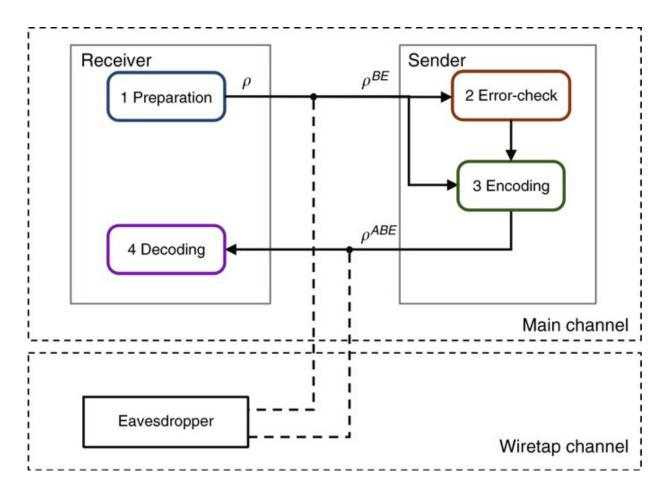
Illustration of the practical DL04-QSDC protocol. The "main channel" and the "wiretap channel" are discrete memoryless channels. The main channel represents a channel between the sender and the legitimate receiver, while the wiretap channel represents a channel between the sender and the eavesdropper. Credit: Light: Science & Applications, doi: https://doi.org/10.1038/s41377-019-0132-3
