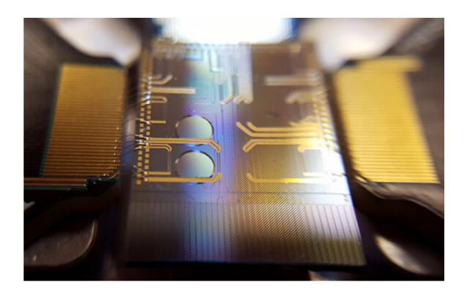
Integrated ring resonator circuitry that is used to generate quantum optical frequency combs. Credit: Swinburne University of Technology
