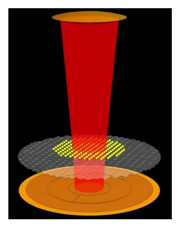
The Quantum Dynamics Unit traps a 2-D layer of electrons in liquid helium, held inside a sealed chamber and cooled to nearly absolute zero. Inside the chamber, a metal plate and spherical mirror on the top reflect microwave light (the red beam), and thus form a microwave cavity (resonator). The trapped microwaves interact with the electrons floating on the liquid helium. Credit:
