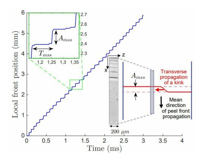
Micro-stick-slip dynamics of the local longitudinal position of the peel front during an experiment at V = 1.8 m/s, L = 50 cm and  $\theta$  = 90°, with periods of rests  $T_{mss}$  preceding slips of size  $A_{mss}$ , as a result of the transverse propagation across the tape of a kinked fracture of amplitude Amss. We also display a typical
