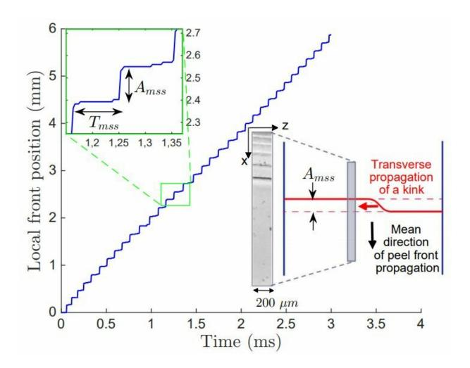
Micro-stick-slip dynamics of the local longitudinal position of the peel front during an experiment at V = 1.8 m/s, L = 50 cm and  $\theta$  = 90°, with periods of rests T<sub>mss</sub> preceding slips of size A<sub>mss</sub>, as a result of the transverse propagation across the tape of a kinked fracture of amplitude Amss. We also display a typical
