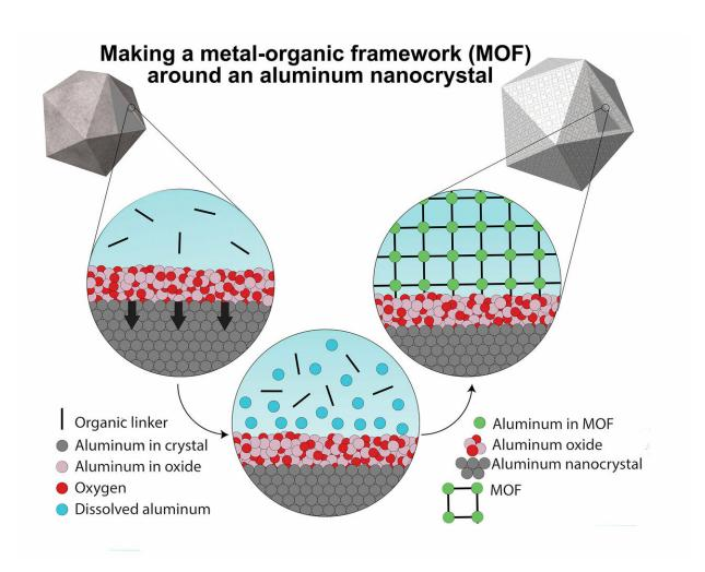
A graphic illustrating the synthesis method that begins with oxide-covered aluminum nanocrystals (top left) and ends with the nanocrystal encased in metalorganic framework (MOF). The MOF self-assembles around the particle when the oxide partially dissolves, releasing aluminum ions that bind with organic linkers to form a 3D framework. (Image courtesy of LANP/Rice University)
