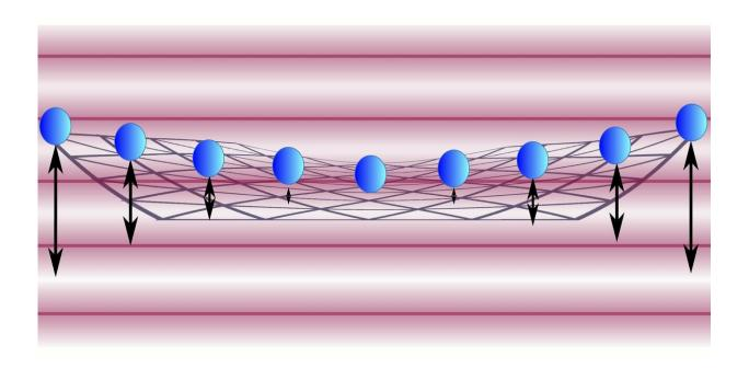
Illustration of vibrating beryllium ions (electrically charged atoms) trapped in a crystal formation. NIST researchers cooled and slowed these 'drumhead' vibrations to nearly motionless. Credit: Jordan/NIST
